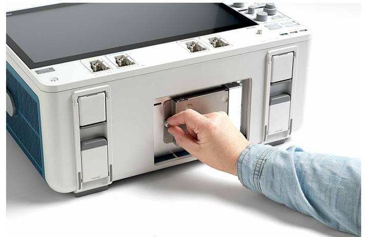
When the SSD is present, the instrument boots in an open Windows 10 configuration, so you can minimize the oscilloscope application and access a Windows desktop where you can install and run additional applications on the oscilloscope or you can connect additional monitors and extend your desktop.
