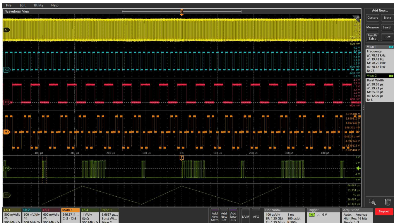
Using measurements to characterize burst width and Frequency.
