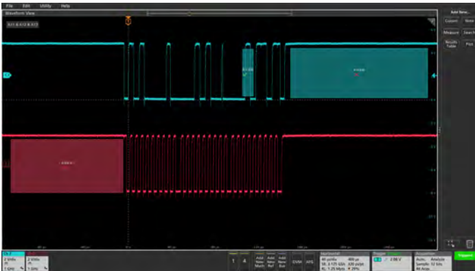
Multiple channel triggering. Visual Trigger areas can be associated with events spanning multiple channels such as packets transmitted on two bus signals simultaneously.
