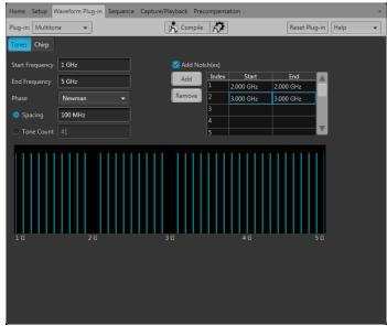
The Tektronix Multitone application plug-in enhances the capabilities of either the AWG70000A Series Arbitrary Waveform Generators or the SourceXpress<sup>®</sup> application software, adding the ability to generate Chirps and Tones.
