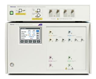
The AWG70000 Series can reach sampling rates as high as 50 GS/s with 10 bits vertical resolution. Such level of performance allows for the direct generation of IQ basebands signals required by modern coherent optical communication systems. The arbitrary waveform generation capabilities of the AWG70000 Series makes it possible to create multi-level signals such as 16QAM, add impairments to a signal, or to create waveforms that are precompensated for the real-world effects of the test system.
