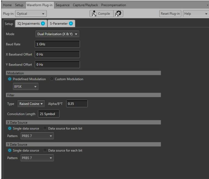
The Tektronix Optical Signals Plug-in is a waveform creation tool that is optimized for the generation of waveforms with complex modulation schemes for the purpose of testing optical communications components and other devices.
