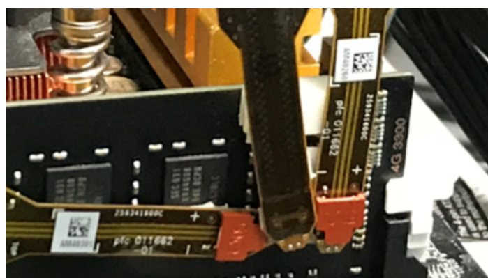
Figure 2: P77STFLXB solder down, flex-circuit accessory provides a probing solution for DDR4 and LPDDR4 electrical validation when used with Nexus XH Series Interposers.
