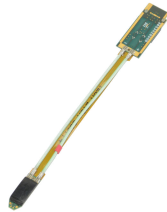
P77STCABL solder down accessory with a long reach, flexible cable combined with an active buffer amplifier on the tip.
