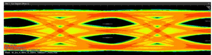
Figure 17: Eye diagram of a three meter cable
