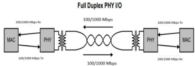
Automotive Ethernet operates as a full-duplex communication link over a twisted pair cable. The full-duplex communication along with PAM3 signaling adds complexity in validating the ECUs in the real world conditions.
