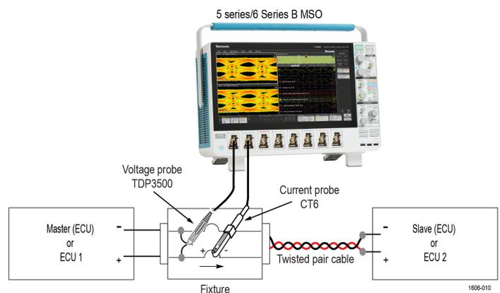
Figure 2: Automotive Ethernet Signal Separation using Fixture
