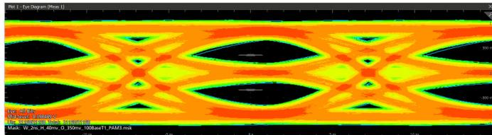
Figure 9: Automotive Ethernet 100BASE-T1 Transmitter Eye diagram
