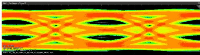
Figure 10: Automotive Ethernet 100BASE-T1 Receiver Eye diagram
