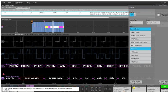
Figure 19: Automotive Ethernet Protocol Decode for full-duplex ECU
