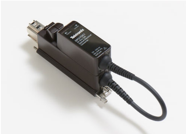
DPO70E1 33 GHz optical probe
