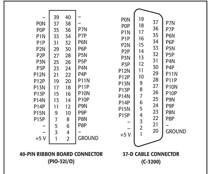
For pin assignments of channels 16-31, add sixteen to the channel numbers shown, (i.e. P0N becomes P16N, etc.)
