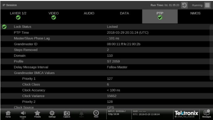
IP Session application showing the PTP lock status and PTP information.
