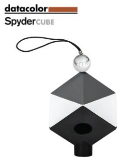
Reference object with specular highlight, 90% white, 18% gray, black, and light trap.
