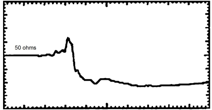
5% rho/div and 200 ps/div. 35 ps TDR of AC port
