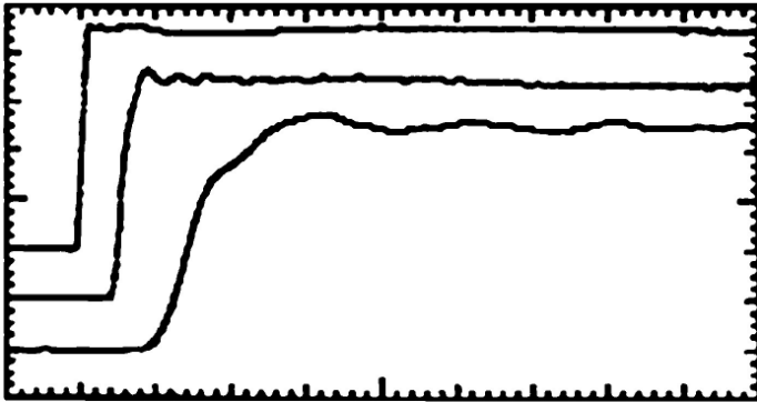
Top to bottom: 500 ps/div, 100 ps/div, and 20 ps/div. 10 ps Step Response
