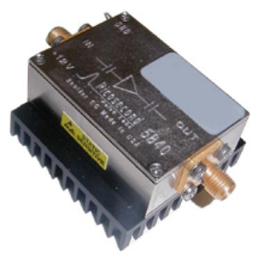
This Ultra-Broadband Amplifier is an excellent choice for either pulse or RF applications. It offers a very attractive price/performance ratio. It is ACcoupled and extremely broadband, covering 5  $\frac{1}{2}$  decades from 80 kHz to 13.5 GHz. It has a clean transient response and smooth gain vs. frequency response. This is a stable 50  $\Omega$  amplifier, and several can be connected in cascade for higher gains.
