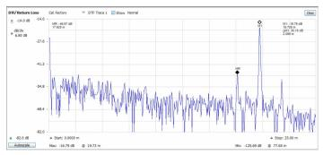
Return loss vs distance for a cable with an inserted barrel and an extension cable. The point at M2 (17.638 m, MR) is the barrel connector and the point marked by M1 at 19.725 m is the end of the cable.
