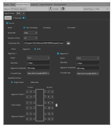
The Tektronix S-Parameters license unlocks the S-Parameter feature available in several of the application plug-ins (available for the AWG70000A Series Arbitrary Waveform Generators or the SourceXpress® application software) adding the ability to apply S-Parameters directly onto a waveform.
