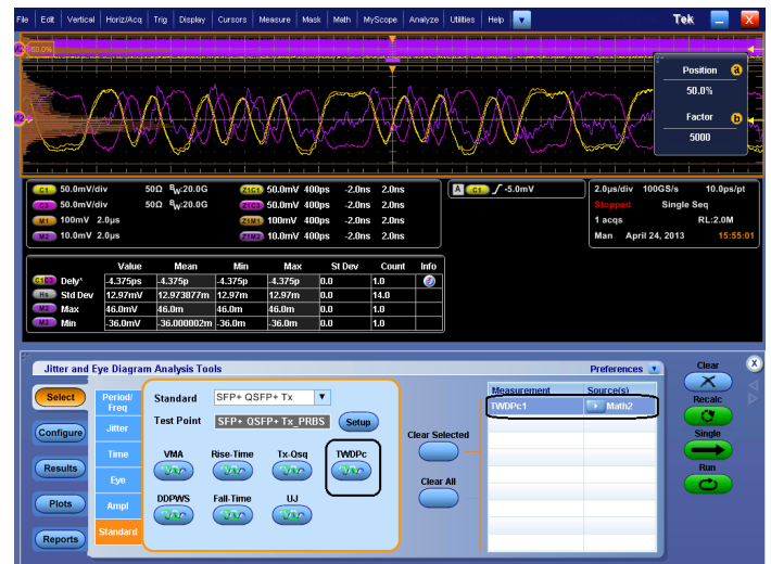
SFP-TX TWDPc measurement – DPOJET user interface.
