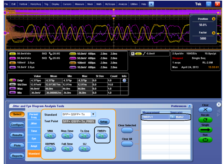
SFP-TX TWDPc measurement – DPOJET user interface.
