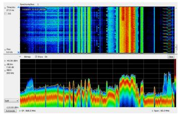
DPX Spectrograms provide gap-free spectral monitoring for up to 12 years at a time. 60,000 traces can be recorded and reviewed, with resolution per line adjustable from  $125 \mu s$  to 6400 s.
