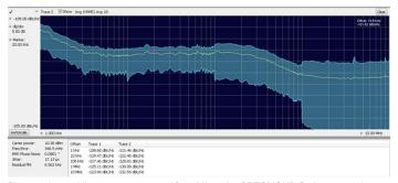
Phase noise and jitter measurements (Opt. 11) on the SPECMONB Series may reduce the cost of your measurements by reducing the need for a dedicated phase noise tester. Outstanding phase noise across the operating range provides margin for many applications. Here, phase noise on a 13 MHz carrier is measured at -119 dBc/Hz at 10 kHz offset. The instrument phase noise of < -134 dBc/Hz at this frequency provides ample measurement margin for the task.
