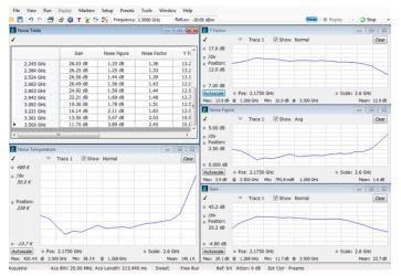
Noise Figure and Gain measurements (Option 14) help you to guickly and easily measure your device using the RTSA and a noise source. This image shows the measurement summary table with graphs of noise temperature, gain, noise figure and Y-
