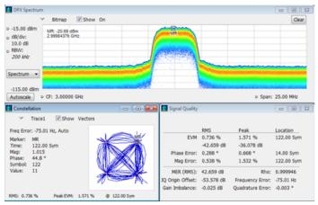
Multiple domain views provide a new level of insight into design problems not possible with conventional analyzers, here, modulation quality and constellation view are combined with the continuous monitoring of the DPX spectrum display.
