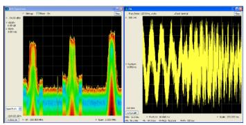
Audio monitoring and modulation measurements simultaneously can make spectrum management an easier, faster task. Here, the DPX spectrum display shows a live spectrum of the signal of interest and simultaneously provides demodulated audio to the internal instrument loudspeaker. FM deviation measurements are seen in the right side of the display for the same signal
