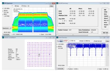
Analysis options for 802.11 standards are available. Here, an 802.11ac 160 MHz bandwidth signal is analyzed, with displays of constellation, amplitude vs. time, summary of WLAN measurements, and the DPX spectrum of the analyzed signal. The density of the 'shoulders' of the WLAN signal are clearly seen in the DPX display, and a marker has been placed on the suppressed center carrier of the signal. An EVM of -47.65 dB and other signal measurements are seen in the summary panel
