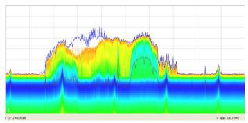
Advanced Triggers, Swept DPX, and Zero Span provides superior swept spectrum analysis for transient signals. Here, a 150 MHz swath of spectrum is swept across the ISM band. Multiple WLAN signals are seen, and narrow signals seen in the blue peakhold trace are Bluetooth access probes. Multiple interfering signals are seen below the analyzers noise level in the multi-color DPX display.
