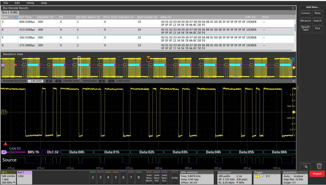
Protocol Decode Results Table provides a time-stamped, tabular view of all captured packets on the CAN FD bus.
