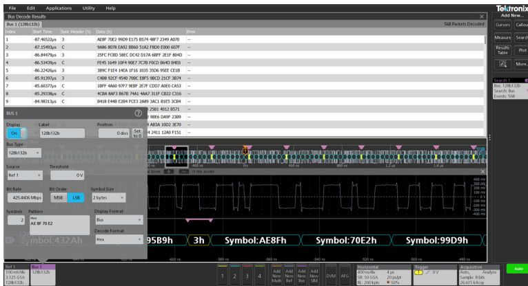
128B132b bus showing decode with LSB. Sync Header was searched with 568 occurrences.
