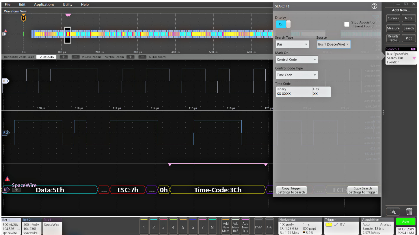
Searching on a specific data pattern on the SpaceWire bus and automatically searching on Sync.
