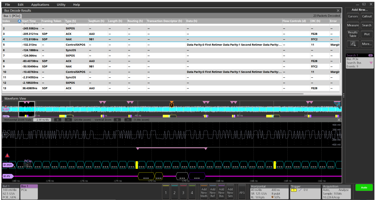
PCIe Gen4 bus showing decode with packet view On. DLP packet of type ACK was searched with 9 occurrences.
