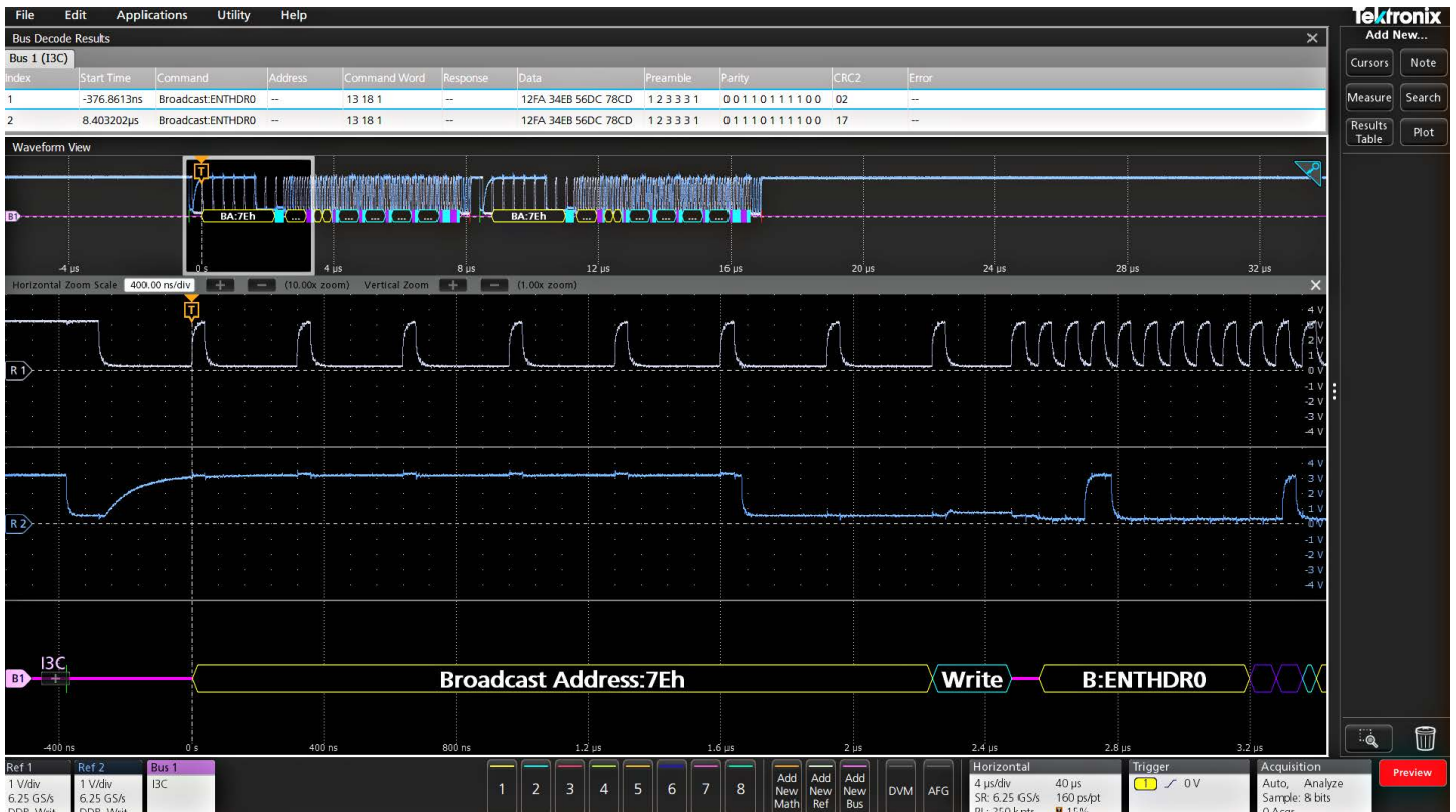
The Protocol Decode Results Table provides a time-stamped, tabular view of all captured packets on the I3C bus.
