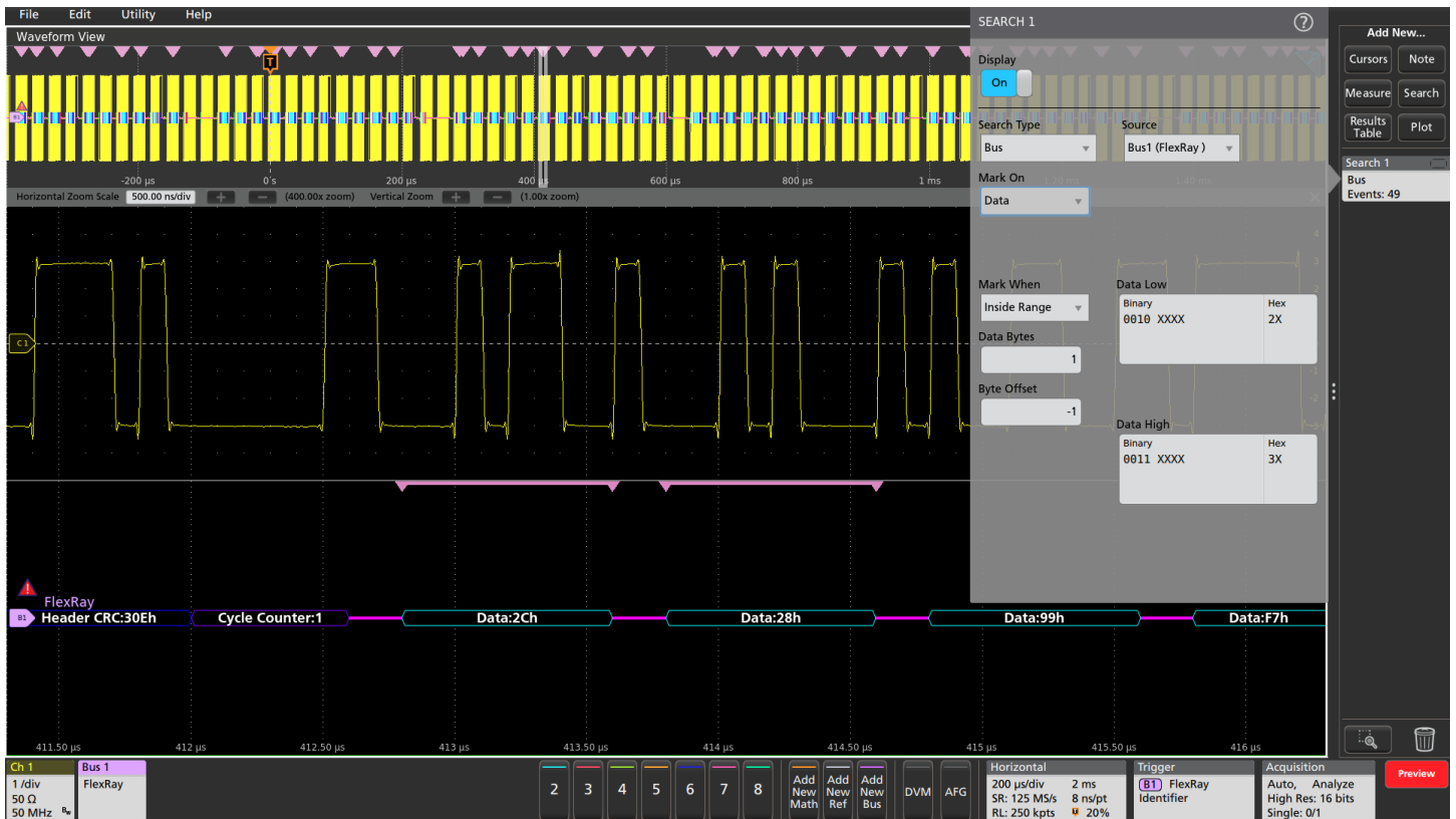
Decoded FlexRay bus, with all data values in a specific range marked with pink brackets.
