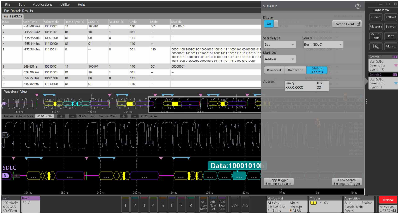
Searching on a station address on the SDLC bus.
