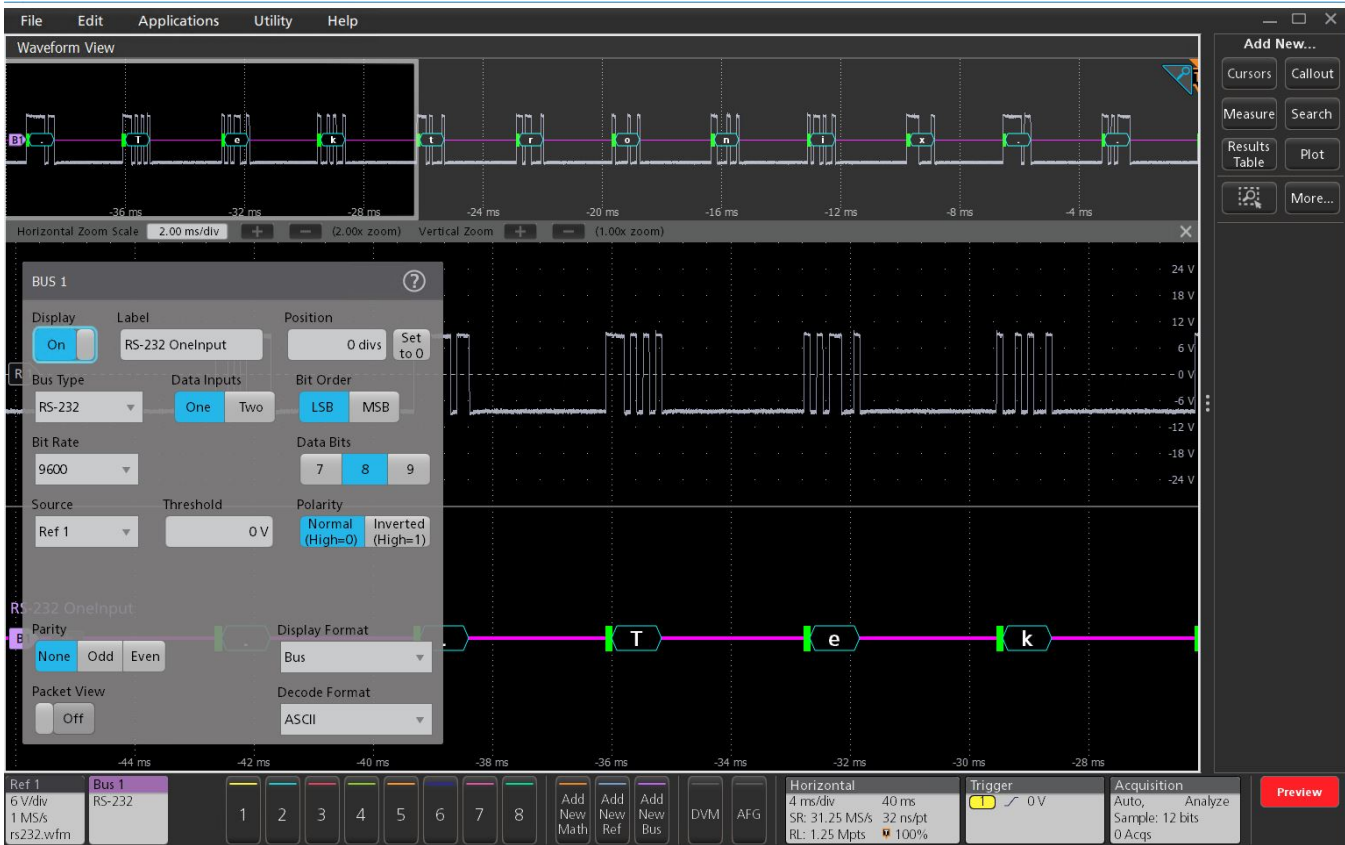
RS-232 bus setup and ASCII display, showing assignment of source signal, digital threshold, and polarity.
