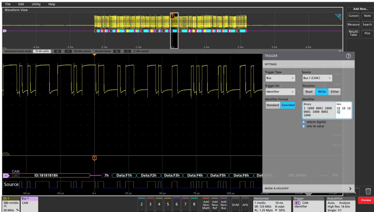
Triggering on a specific extended Identifier value on the CAN bus.
