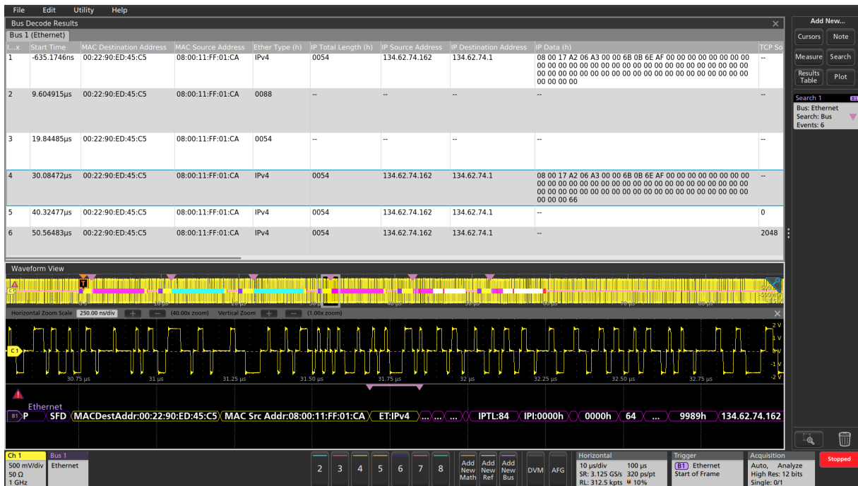
Triggering and automatically searching on the 100BASE-TX Ethernet bus.
