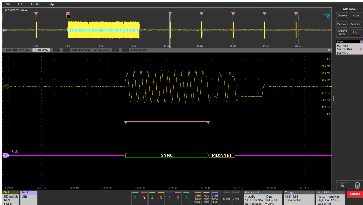
Triggering on a specific data pattern on the USB 2.0 bus and automatically searching on Sync.
