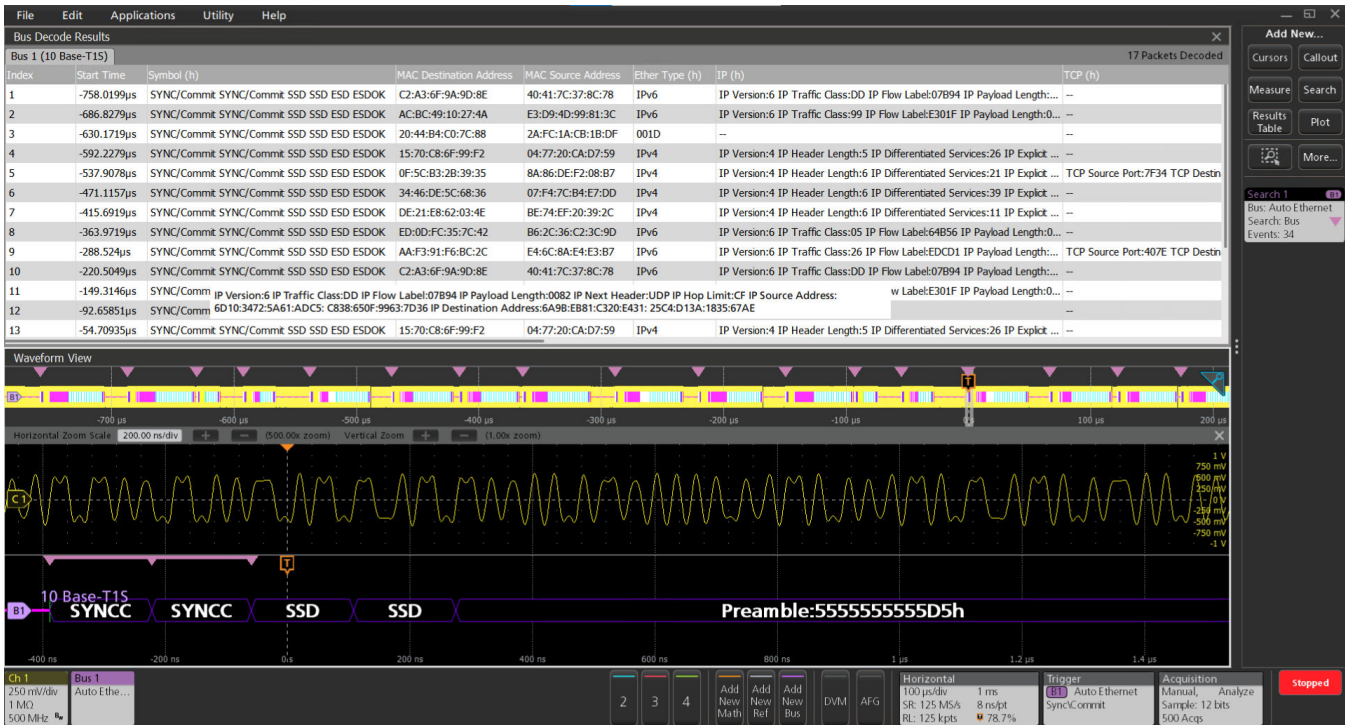
10BASE-T1S bus decode and results table in a tabular format. Searching the 10BASE-T1S bus decode with search on Sync/Commit with 34 occurrences shown on the search badge.
