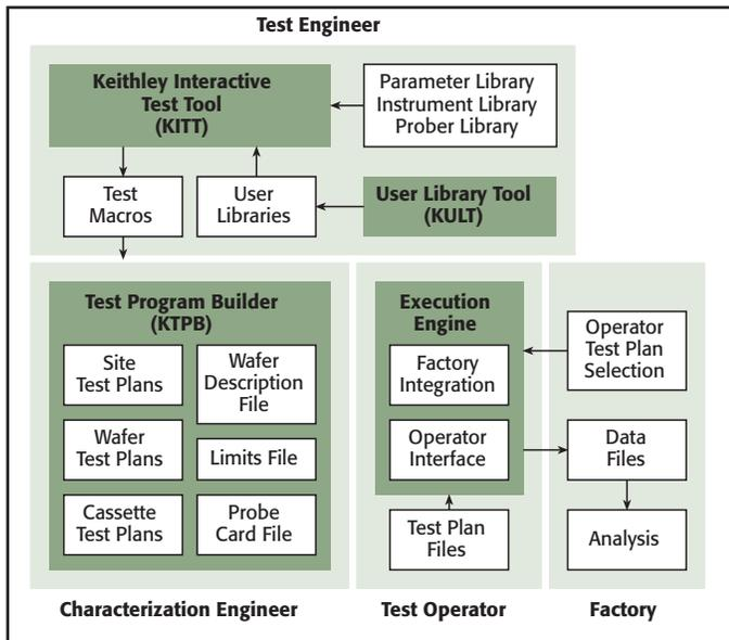
Figure 3. KTE software architecture
