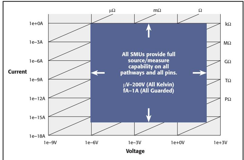
Figure 1. Series S600 measurement ranges
