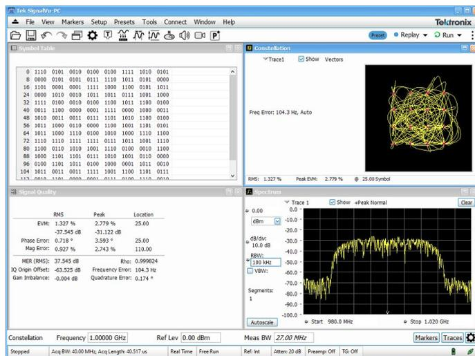
Wideband satellite and point-to-point microwave links can be directly observed with SignalVu-PC analysis software. Here, general purpose Digital Modulation Analysis (SVM) is demodulating a 16QAM backhaul link running at 312.5 MS/s.
