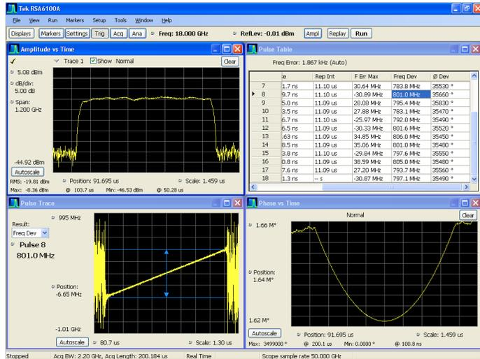
The Advanced Signal Analysis package (Opt. SVP) provides 27 individual measurements to automatically characterize long pulse trains. An 800 MHz wide LFM chirp centered at 18 GHz is seen here with measurements for pulses 7 through 18 (upper right). The shape of the pulse can be seen in the Amplitude vs. Time plot shown in the upper left. Detailed views of pulse #8's frequency deviation and parabolic phase trajectory are shown in the lower two views.
