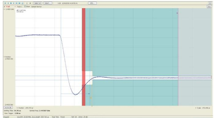
Settling time measurements (Opt. SVT) are easy and automated. The user can select measurement bandwidth, tolerance bands, reference frequency (auto or manual), and establish up to 3 tolerance bands vs. time for Pass/Fail testing. Settling time may be referenced to external or internal trigger, and from the last settled frequency or phase. In the illustration, frequency settling time for a hopped oscillator is measured from an external trigger point from the device under test.
