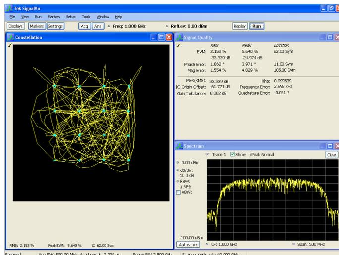
Wideband satellite and point-to-point microwave links can be directly observed with SignalVu analysis software. Here, General Purpose Digital Modulation Analysis (Opt. SVM) is demodulating a 16QAM backhaul link running at 312.5 MS/s.
