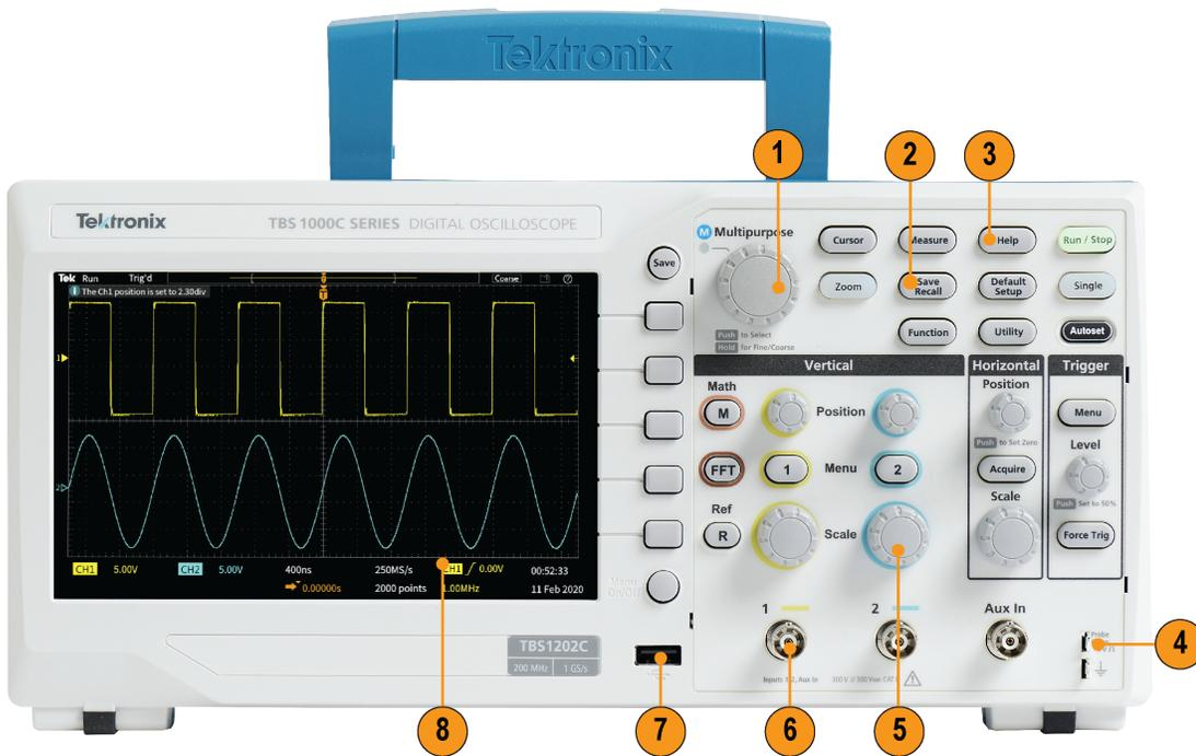
Figure 1: TBS1000C front panel
