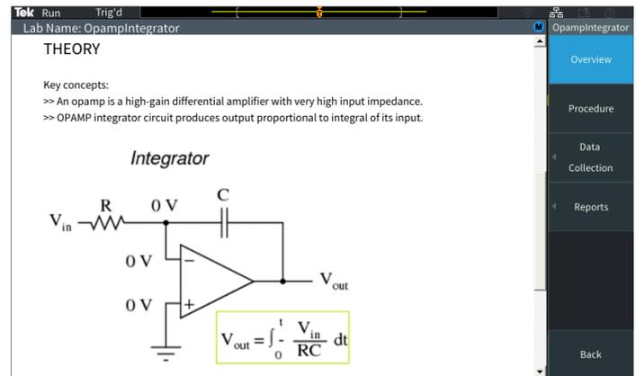
Figure 10: The Courseware function allows students to see lab information on the instrument display
