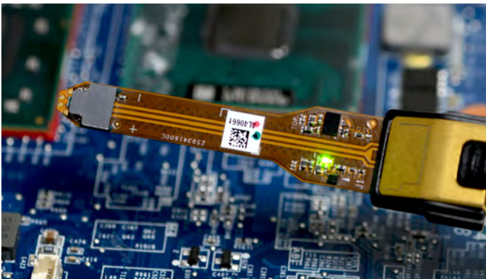
Figure 1: P77STFLXA solder down, flex-circuit accessory with an active buffer amplifier on its tip.
