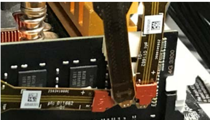
P77STFLXB solder down, flex-circuit accessory provides a probing solution for DDR4 and LPDDR4 electrical validation when used with Nexus XH Series Interposers.
