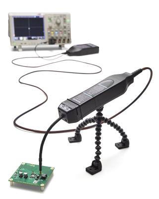
The Tektronix TIVM and TIVH Series IsoVu<sup>™</sup> Measurement Systems offer galvanically isolated measurement solutions for accurately resolving high bandwidth, differential signals up to ±2500 V in the presence of large common mode voltages with the best in class common mode rejection performance across its bandwidth.
