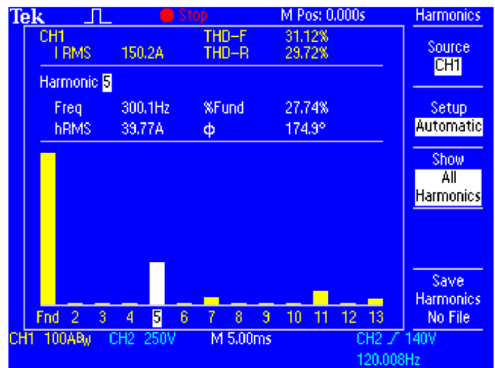
Conduct harmonic distortion measurements with TPS2PWR1 software.
