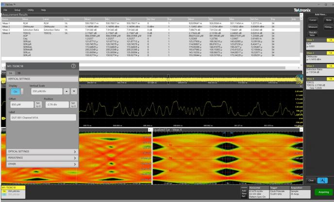
Add reference waveforms for offline processing of previously captured data, view eye diagrams before and after TDECQ FFE equalization, and detach windows from the base software to be rearranged or resized
