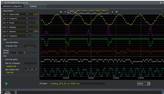
TekBench™ is PC software that controls Tektronix oscilloscopes and arbitrary function generators. It offers intuitive instrument control, automated measurement data logging, automated frequency response measurements, and easy waveform exporting with required format to eliminate extra time and effort. It allow you to focus on their experiment rather than learning the instrument.
