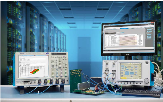
Figure 16: PCIe receiver test setup
