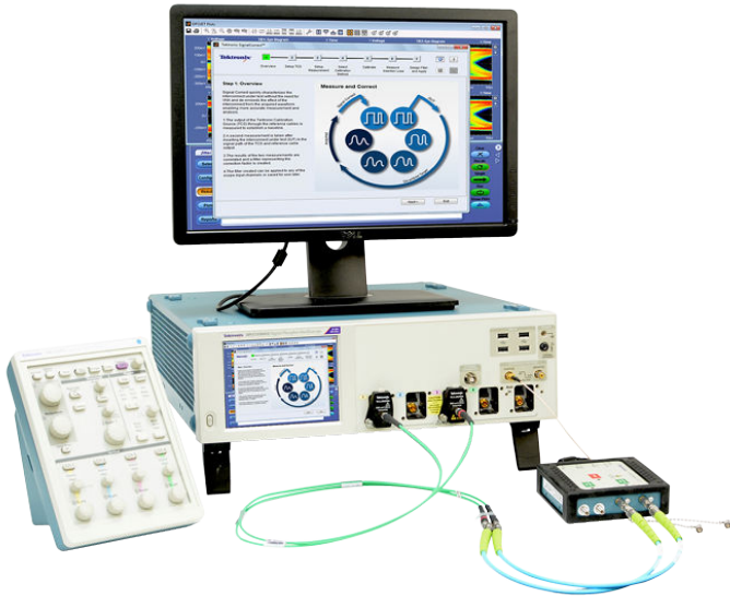
Figure 14: SignalCorrect allows quick characterization of cables, fixtures and other types of interconnects using the TCS70902 fast step source and the response captured on a DPO70000SX Series real-time oscilloscope.
