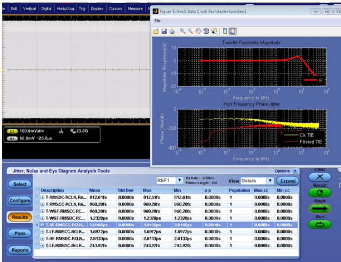
Figure 12: Example of RefClk measurements, together with generated plots
