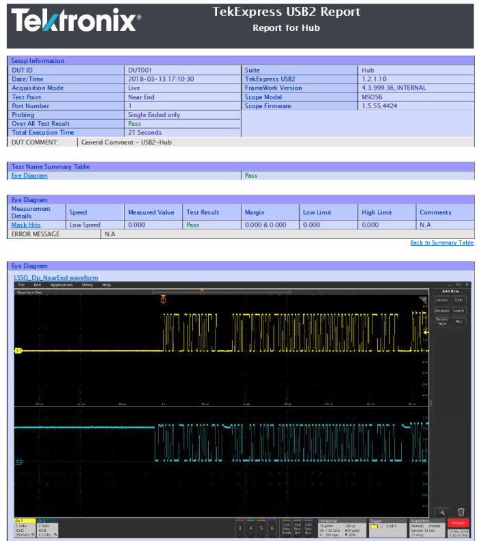
TekExpress USB2 report showing setup details and measurement results
