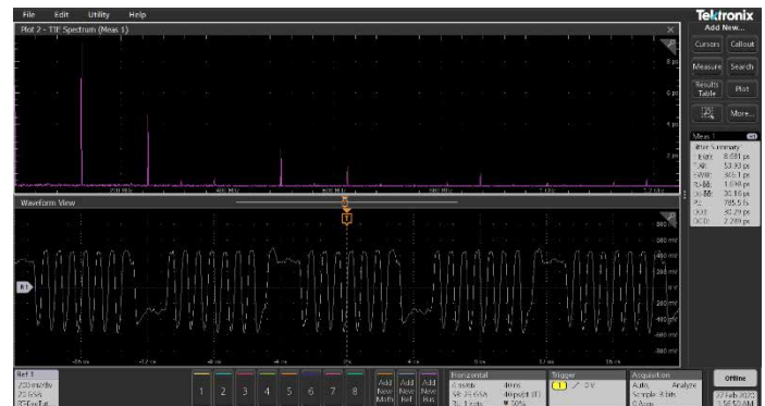
Stacked view of time domain waveform and jitter spectrum
