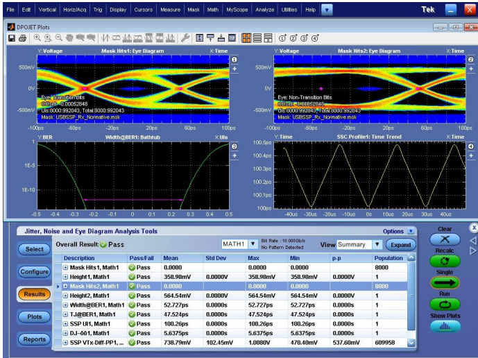
DPOJET Analysis plots displaying eye mask hits, bath tub curve, and SSC profile
