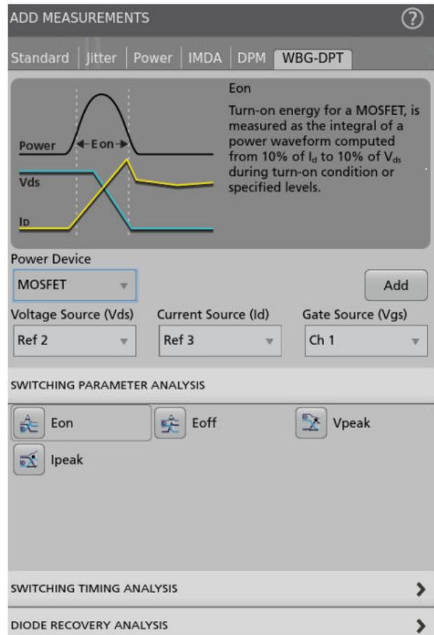
Switching parameter analysis measurements
