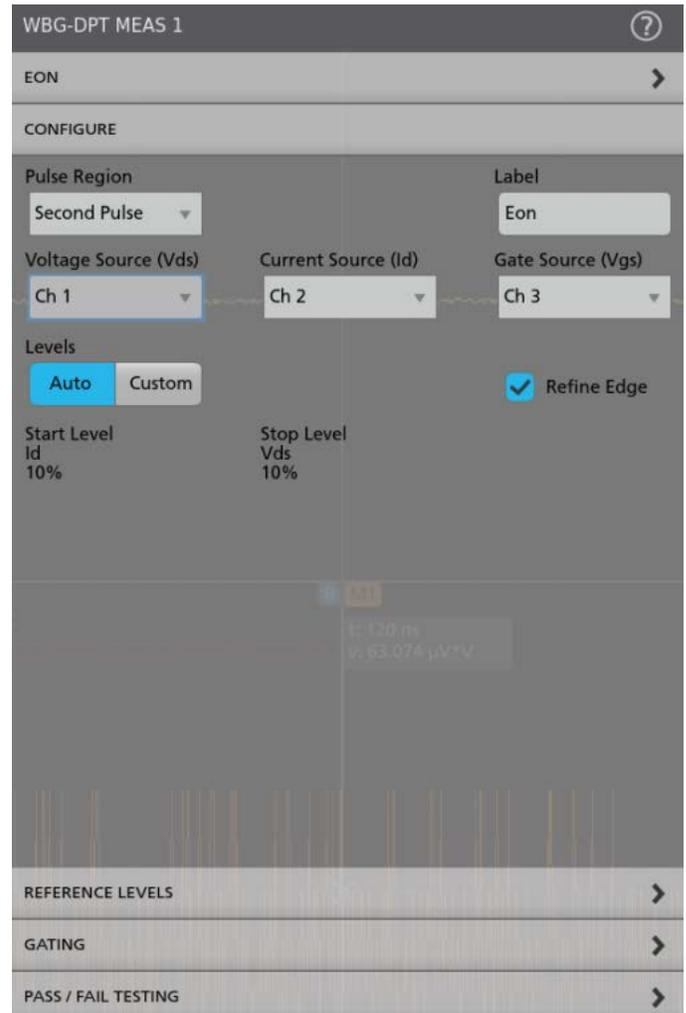
By default, the pulse region is defined as per the standard. For example, Eon in DPT is measured on the second pulse and Eoff is measured on the first pulse. However, you can configure the pulses as per your custom requirements. You can also choose the multiple pulse configuration to test more than two pulses. This offers greater flexibility based on the designs.
