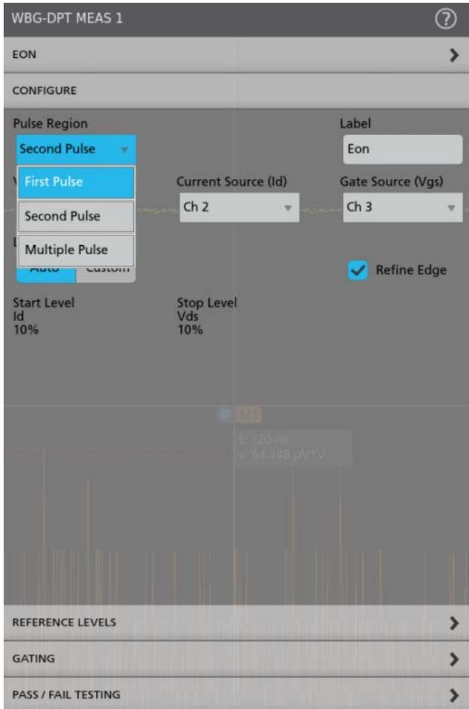
During this operation, it is important to measure the turn-on and turn-off switching parameters of multiple edges. Multiple pulses are supported as part of the measurement configuration.
