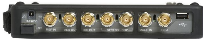
WFM2200A top panel connectors.
