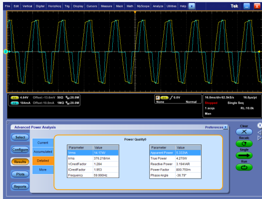
AC power analysis using DPOPWR on an MSO5000B oscilloscope
