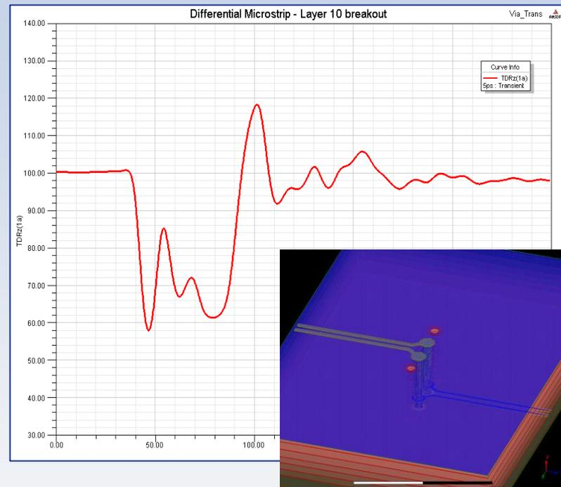
**Note: A non-optimal antipad size is used to dramatize the reflection from the via transition in the animation**
