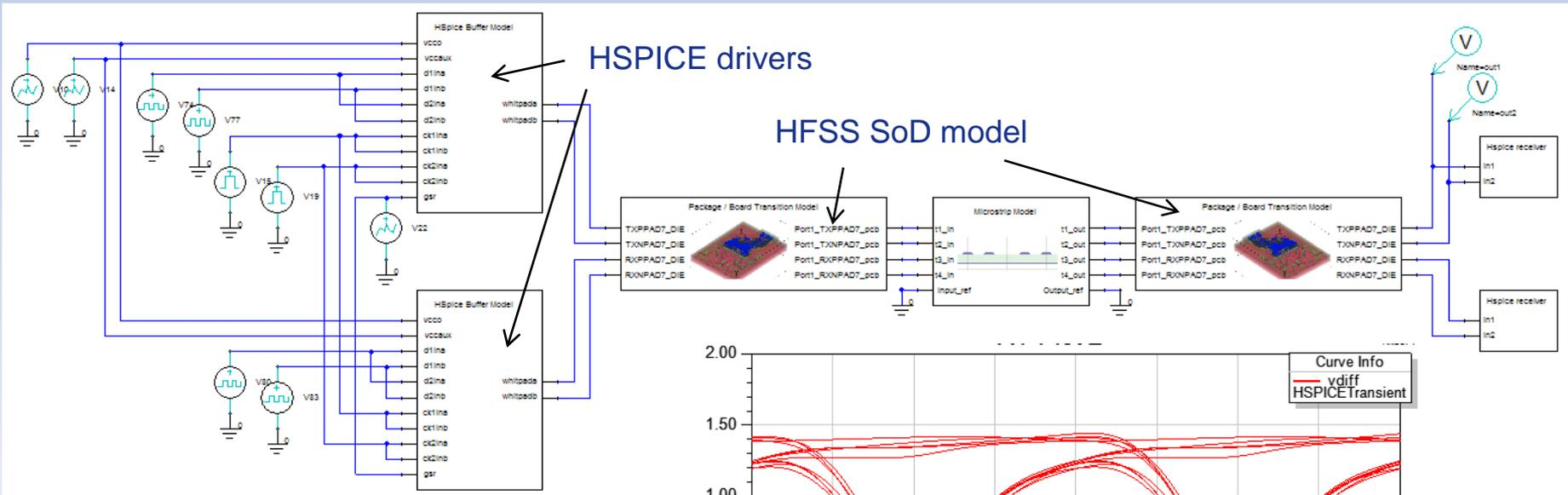
Complex transistor-level models can result in substantial run times for long bit patterns.
