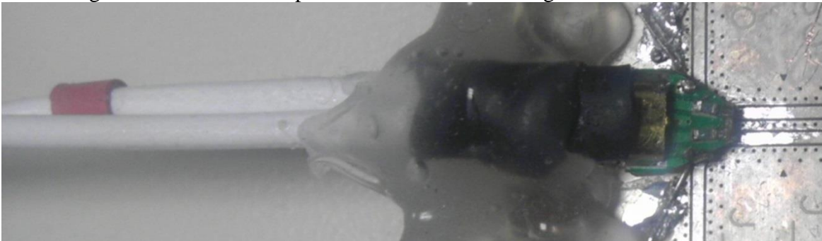
Figure 15: A Soldered 25 GHz Differential Oscilloscope Probe
