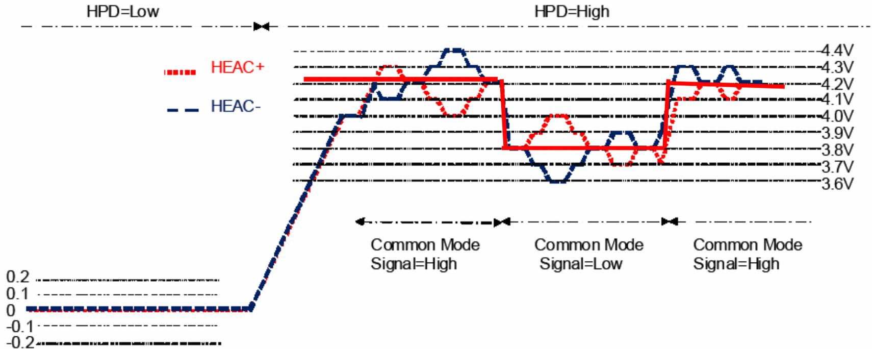
HEAC Figure 2-10 Simultaneous Transmission Waveform
