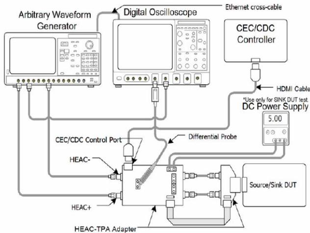
Setup 31. Test ID HEACT 5-16 : Differential Signal Receiver Performance Test-Tektronix
