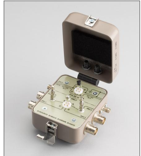
**8101-PIV:** DC and pulse I-V demo fixture that is a metal case with four female triax connectors, two SMA connectors, and a latch. Inside the test fixture are two 4-pin device holders (transistor sockets) and two plungers for parts with two leads.
