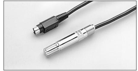
**6517-RH Humidity Probe:** The 6517-RH comes with a 3 m (10 ft) extension cable and is designed to be used with the 6517B Electrometer. The 6517-RH measures the relative humidity of the testing environment.
