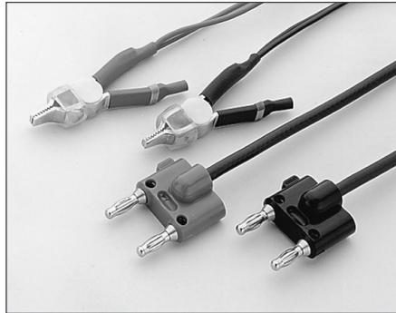
**5806 Kelvin Clip Lead Set:** 2 clip test leads, red and black, 0.9 m (36 in) with banana plug termination. Designed to be used with Keithley instruments that measure 4-terminal resistance. Maximum jaw opening ½ in. A package of 8 replacement elastic bands (P/N 5806-306B) is available.
