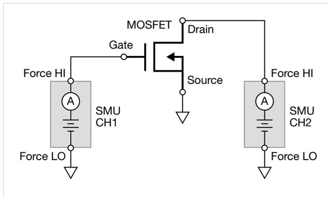
Figure 3. MOSFET test configuration using two SMU channels
