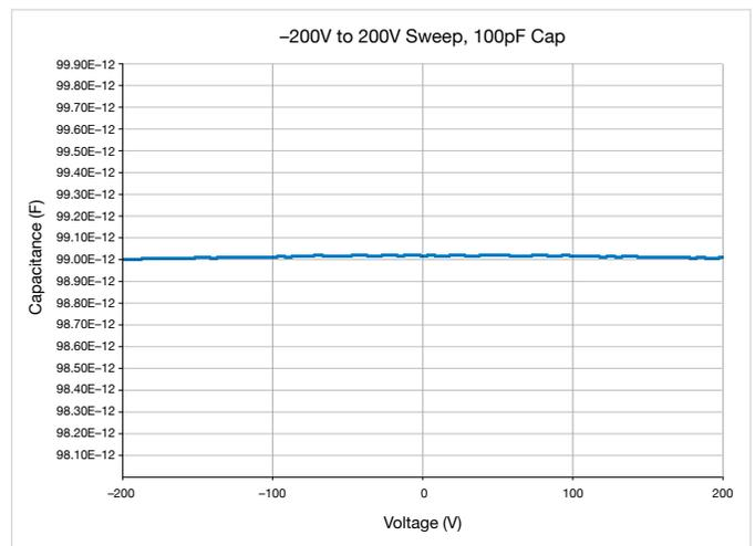
Figure 9. ±200 C-V Sweep on 100pF Capacitor
