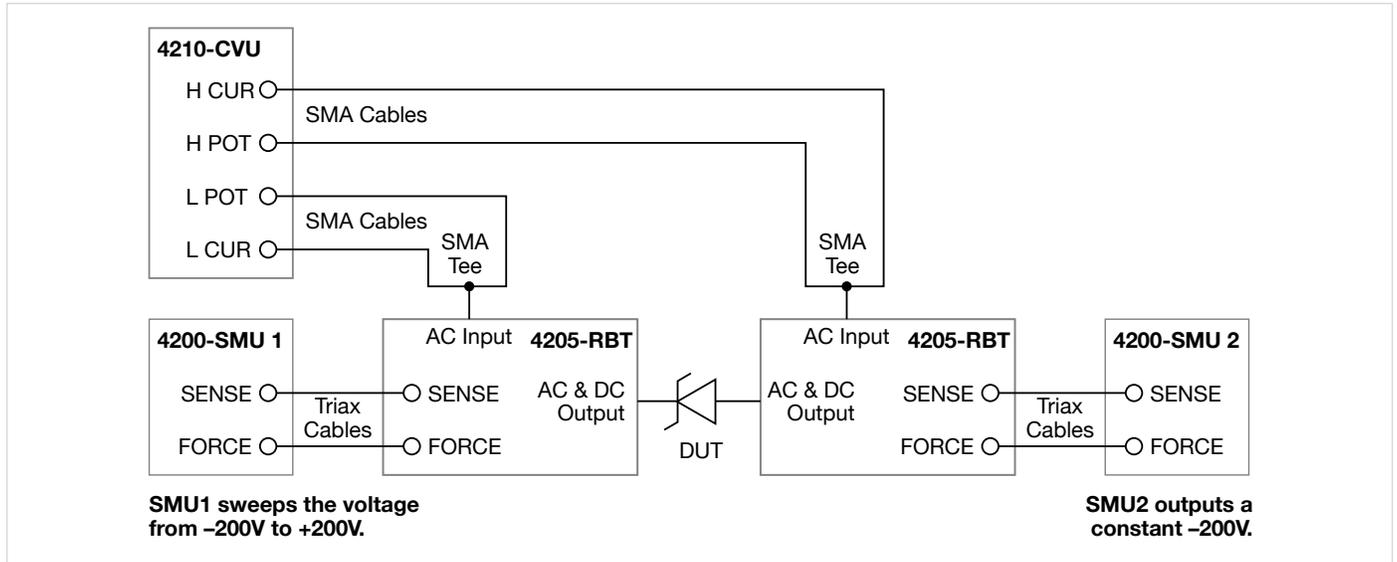
Figure 10. High Voltage C-V Connections for Schottky Diode Test
