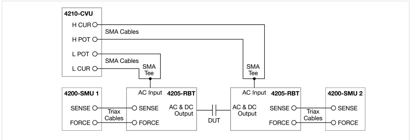
Figure 2. High Voltage C-V Measurements Using Two Remote Bias Tees
