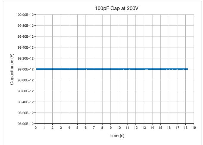
Figure 8. Capacitance vs. Time Measurements
