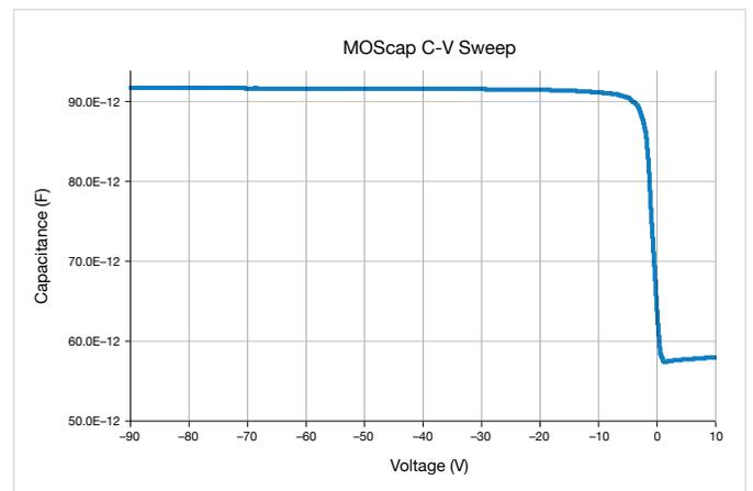
Figure 7. High Voltage C-V Sweep of MOScap
