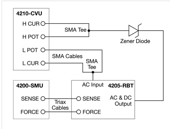
Figure 4. High Voltage C-V Connections for Zener Diode
