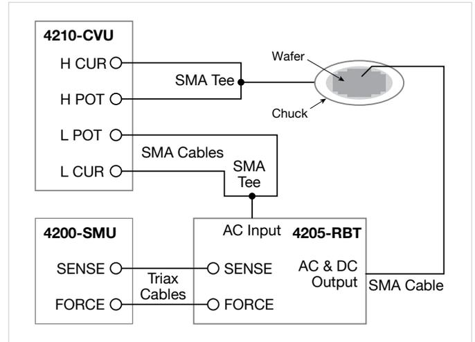
Figure 6. High Voltage C-V Connections for MOScap Testing
