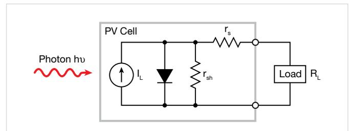
Figure 2. Idealized equivalent circuit of a photovoltaic cell
