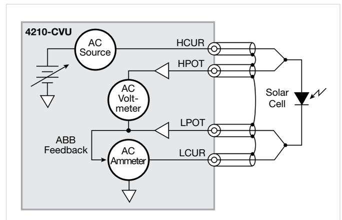
Figure 11. Connecting the solar cell to the 4210-CVU capacitance meter
