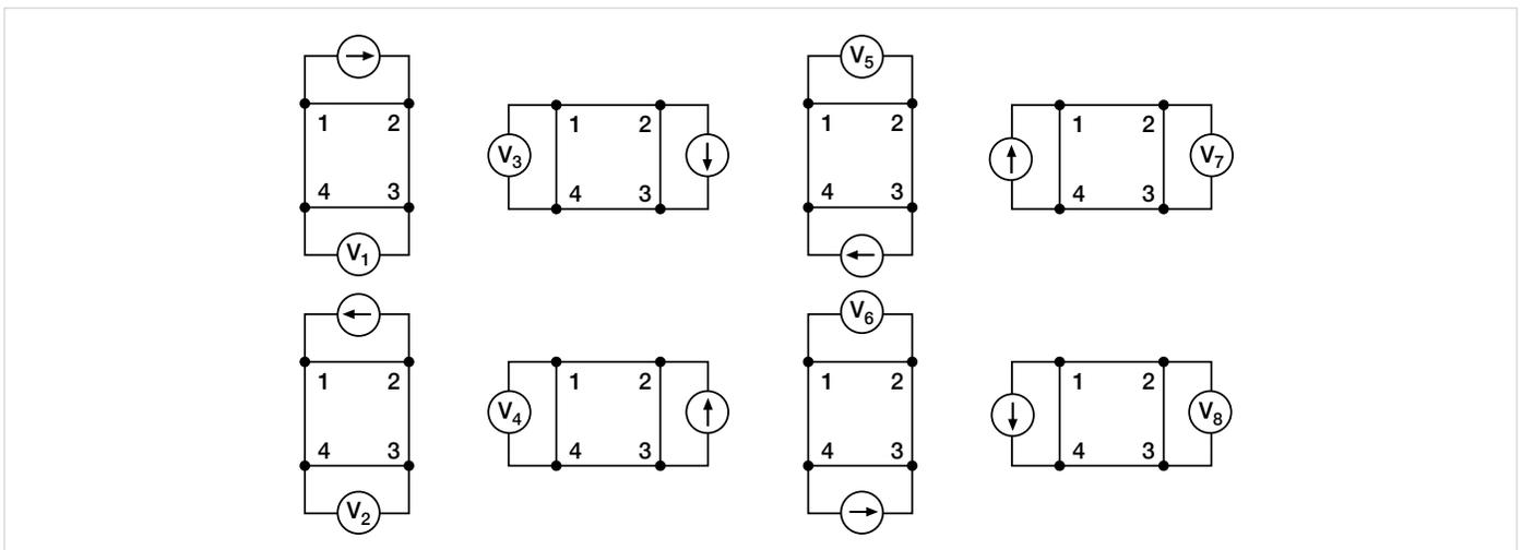
Figure 22. van der Pauw resistivity measurement conventions
