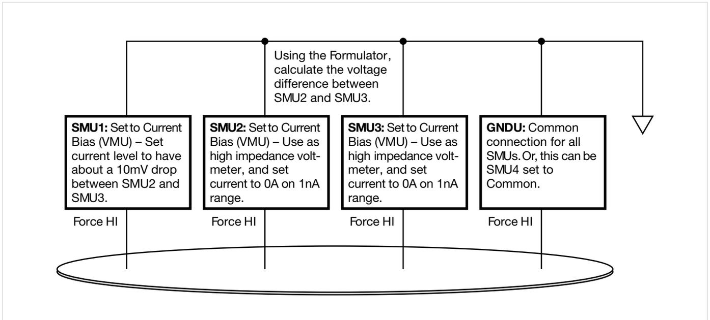
Figure 20. SMU designation for four-point collinear probe measurements
