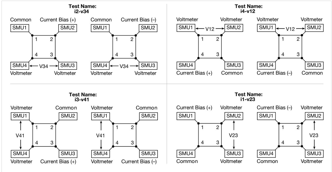
Figure 25. SMU configurations for van der Pauw measurements
