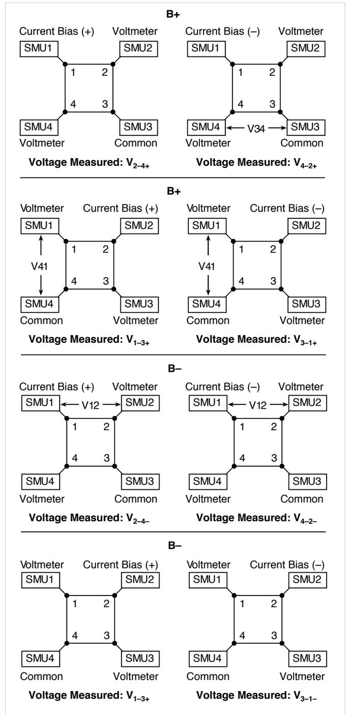
Figure 28. SMU configurations for Hall voltage measurements
