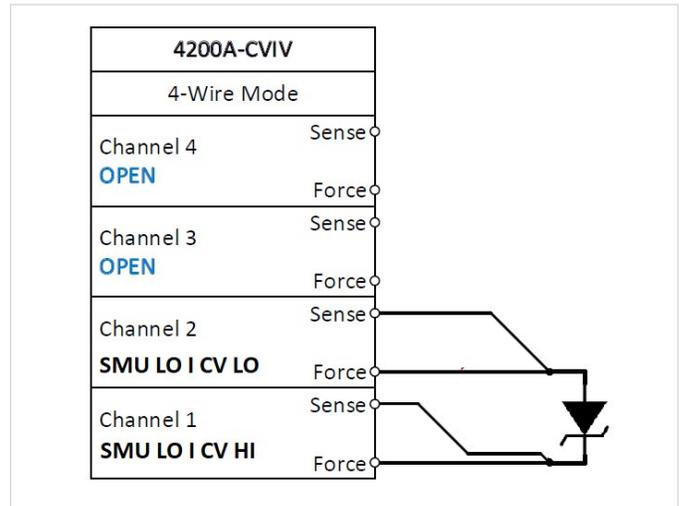
Figure 2: High Voltage C-V Connections for Zener Diode using the CVIV
