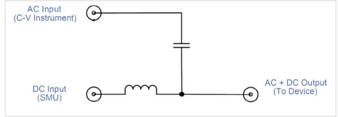
Figure 1: Typical Bias Tee Block Diagram
