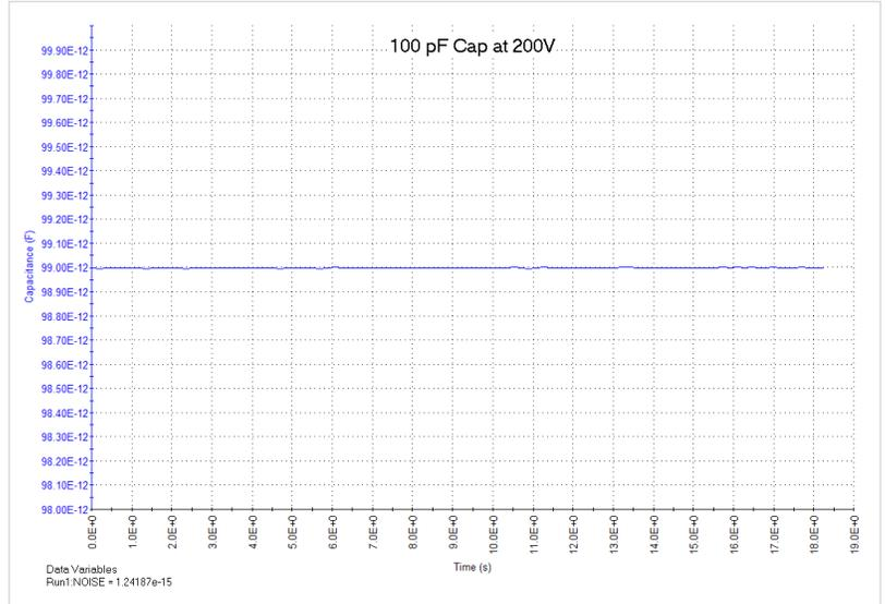
Figure 13: Capacitance vs. Time Measurements
