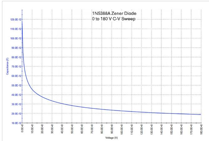
Figure 12: Results of C-V Sweep of Zener Diode
