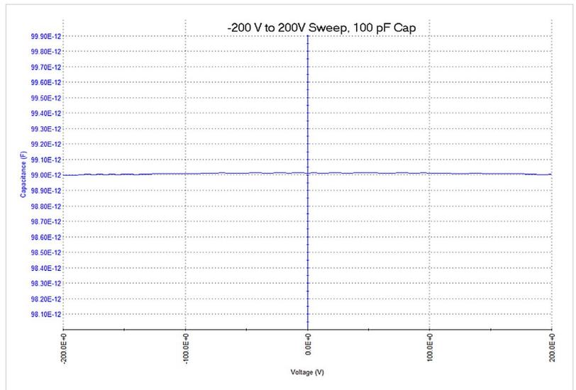
Figure 14: ±200 V Sweep on 100 pF Capacitor
