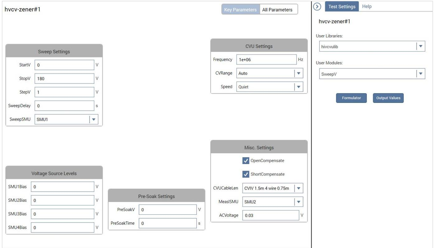
Figure 11: SweepV user Module for High Voltage CV measurement
