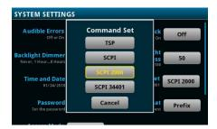
The DMM6500 emulates the Keithley 2000 and Keysight 34401A, so there's no need to change your existing test code.
